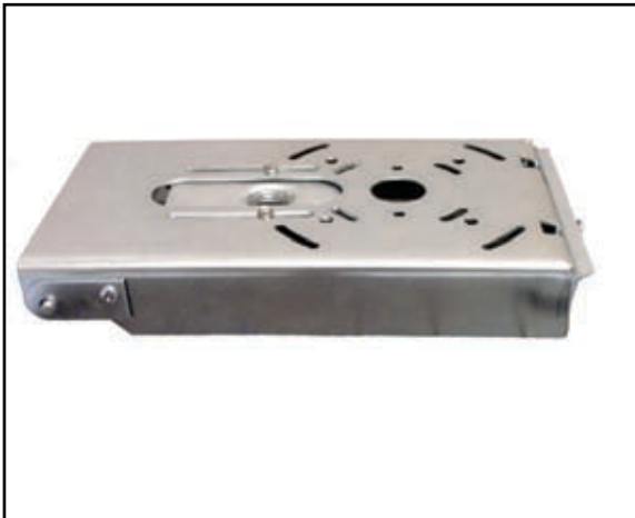
Hinged Quick-Mount Bracket, Stamped Steel, Mount Over Recessed Electrical Box, or Use 3/4" NPS Downrod for Pendant Mounting
